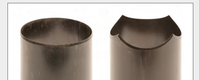
Outside sharpened: push up native soil
